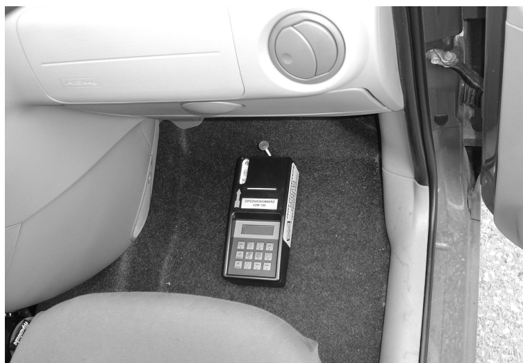
Fig. 3. Decelerometer VZM100 used in investigations
