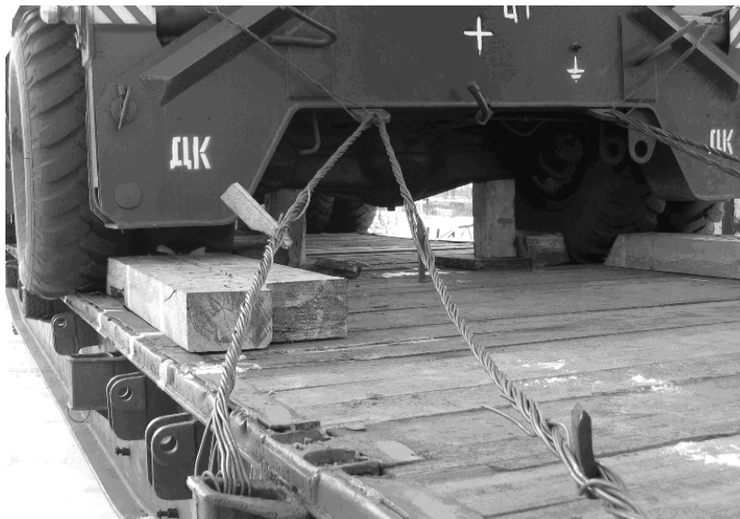
Fig. 2. Weakening of fastening flexible elements of wheel machinery
