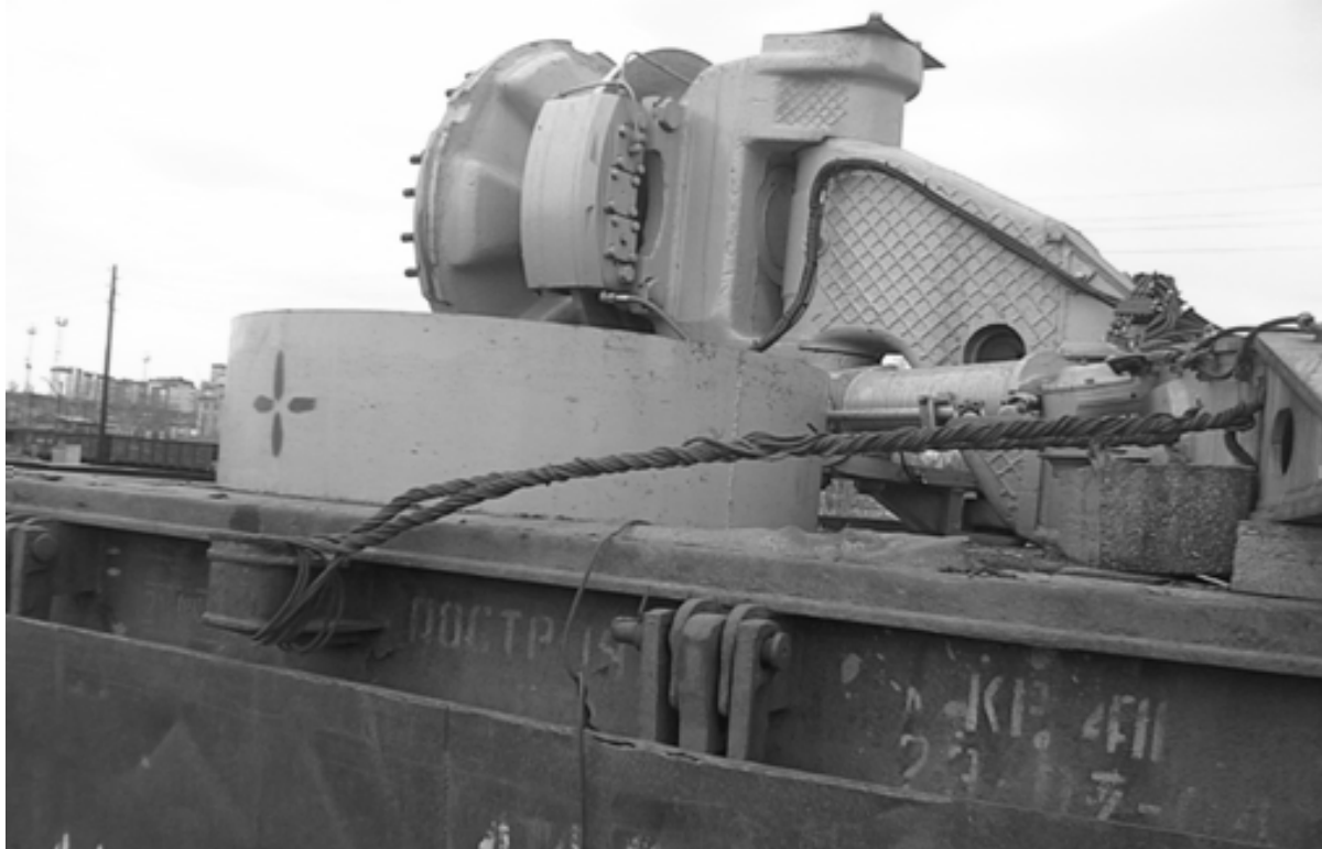
Fig. 4. Loss of constraint of flexible fastening elements of the opposite direction under the exposure to crosswise forces
