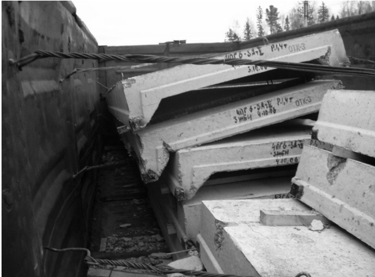
Fig. 3. Illustration of crosswise forces effect manifested in break-up (displacement) of the cargo crosswise the wagon
