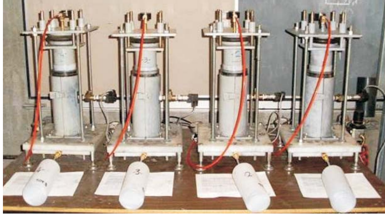
Fig. 1. A series of one-dimensional consolidation tests conducted on CPB samples being cured for 0, 1, 3 and 7 days
