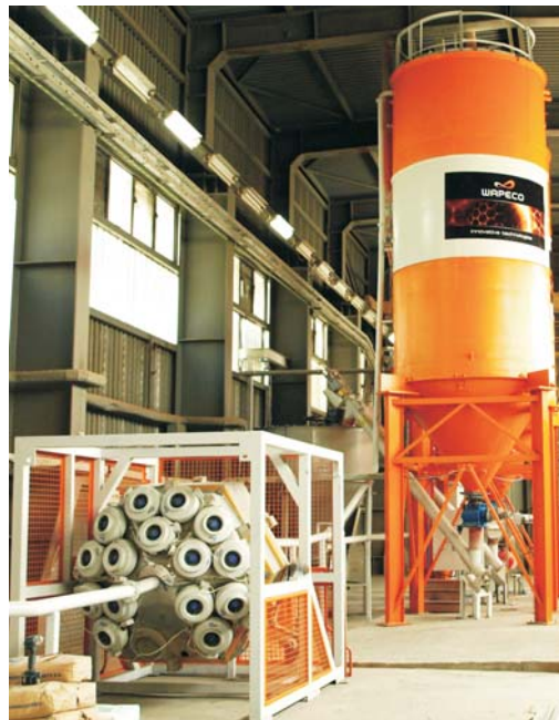
Fig. 1. Wapeco magnetic activator (Widuch et al. 2011a)
