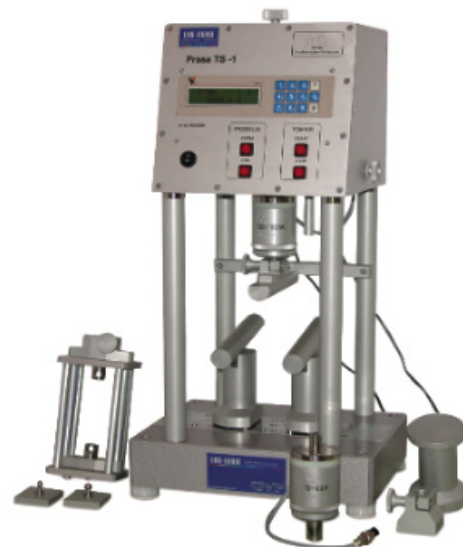
Fig. 4. The stand for bending tests [15]
