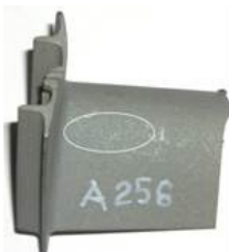
Fig. 14. General view of a fragment of the cast blade with marked places where the defects have occurred
