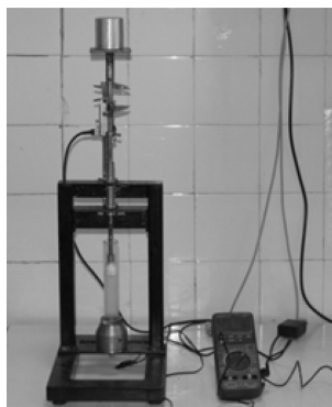
Fig. 2. Experimental stand for testing the wax mixtures shrinkage
