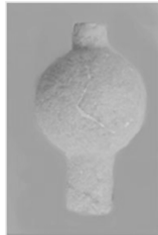
Fig. 8. Technological test of assessment of the ceramic mould cracking tendency during investment casting
