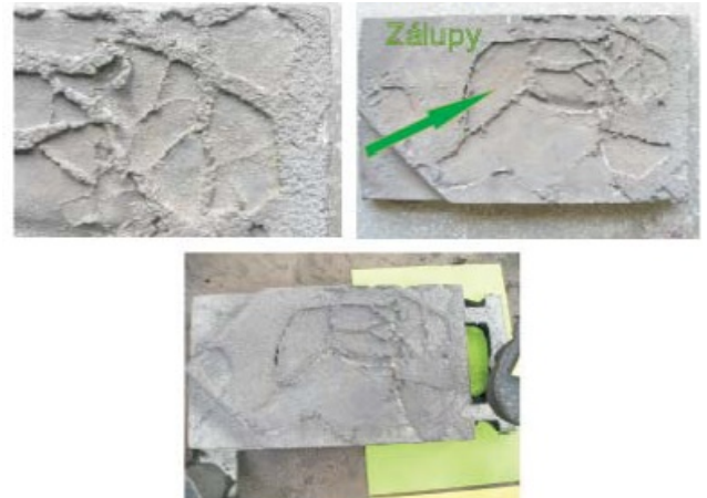
Fig. 10. Test casting - pattern mixture 3
