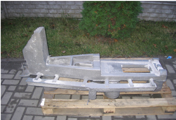
Fig. 4. Casting of the base weighing 102 kg. GJS 400-15
