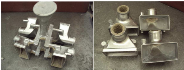
Fig. 8. The knocked out shell and castings separated from the gating system
