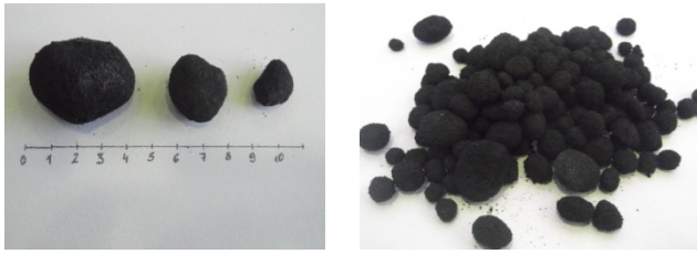
Fig. 3. Granulate fractions, granulator rotational speed – 10 rpm, angle of inclination – 40°, scale in cm
