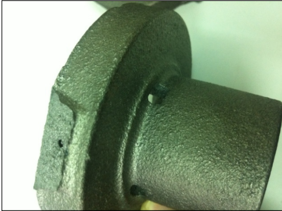
Fig. 6. Shrinkage in the cross-section of the casting and under the feeder
