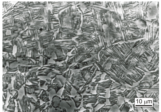
Fig. 6. Microstructure on the border RZ and HAZ
