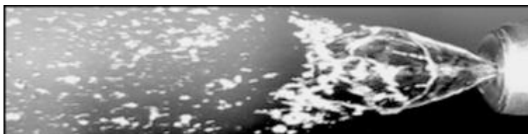
Fig. 5. Generating droplets by the swirl jet, with use of water flow 0.03 l/min and water pressure 0.01
