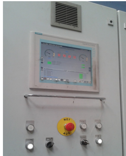
Fig. 4. The control cabinet with a touch screen for setting the sintering process parameters
