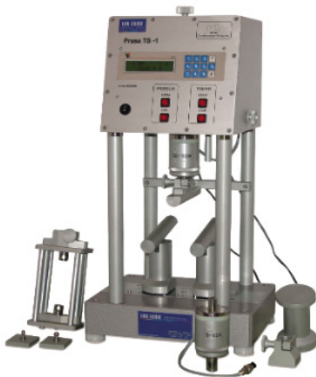
Fig. 7. The stand for bending tests [14]
