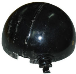
Fig. 1. The container fragment from the steel 30HGS after sample cutting
