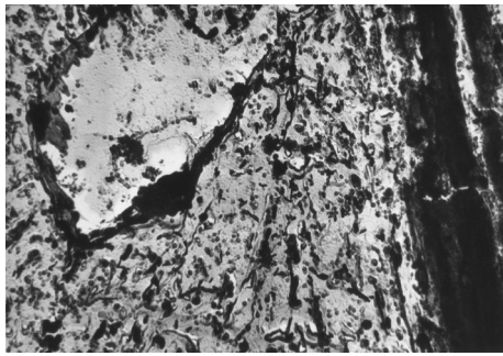
Fig. 8. SiO 2 -CaO-MnO multiphase inclusions deformed during processing. Process (KP). Mag. 10 000x
