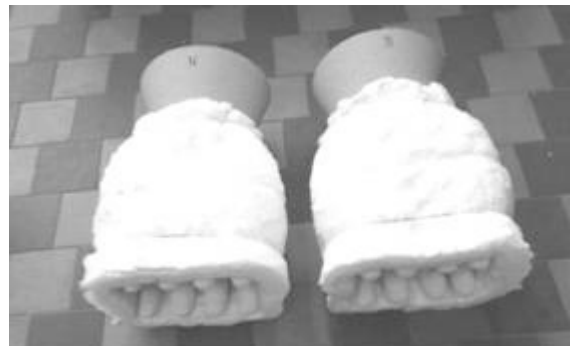
Fig. 3. Moulds with insulation ready for tests
