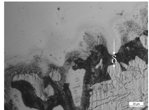
Fig. 7. Microstructure of joint area between austenitic alloy steel and ferritic-pearlitic unalloyed cast steel at C = 0,60% and T_{zal} = 1650^{\circ}\text{C} – etching Mi19Fe
