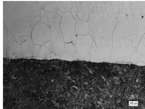
Fig. 6. Microstructure of joint area between austenitic alloy steel and ferritic-pearlitic unalloyed cast steel C = 0,55% at T_{zal} = 1600^{\circ}\text{C} – etching Mi19Fe
