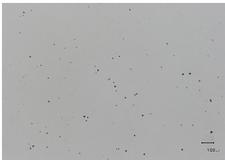
Fig. 5. Globular inclusions after deoxidation with Al+Ti (100 x)
