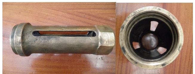
Fig. 1. Casting of safety inlay for steam locomotive
