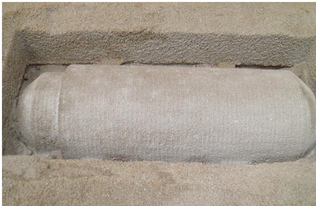
Fig. 11. Core just before removing from the mould
