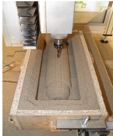
Fig. 10. Milling the core, roughing
