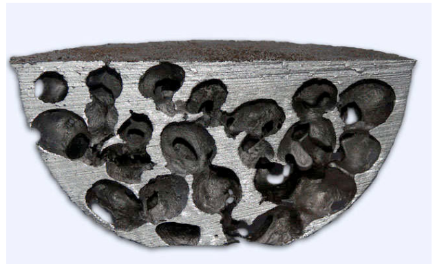
Fig. 4. Open pore casting (organic precursor removed by annealing) VSB-TU Ostrava [5]
