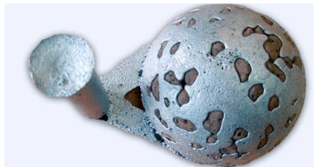
Fig. 5. Open pore casting before annealing VSB-TU Ostrava [5]
