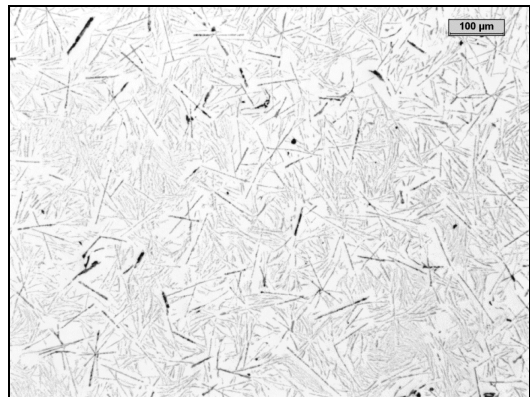
Fig. 4. Microstructure of the aluminium cast iron [own research]
