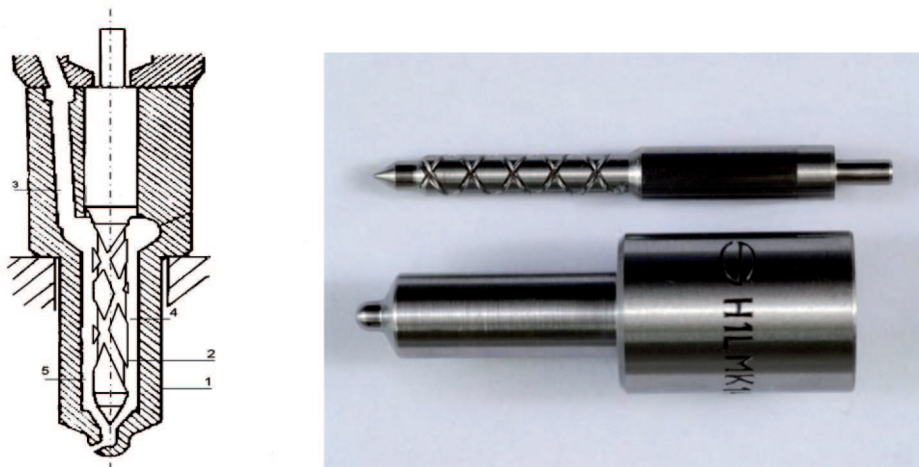
Fig. 2. Diagram and image of a multi-hole injector with the preliminary thermal-catalytic-turbulizing treatment of fuel
