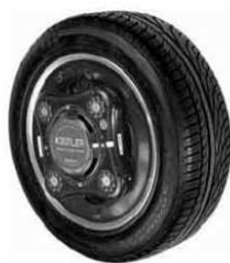
Fig. 2. An example of 6-component strain gage measuring a wheel for passenger vehicles, light weight carbon fiber design [1]
