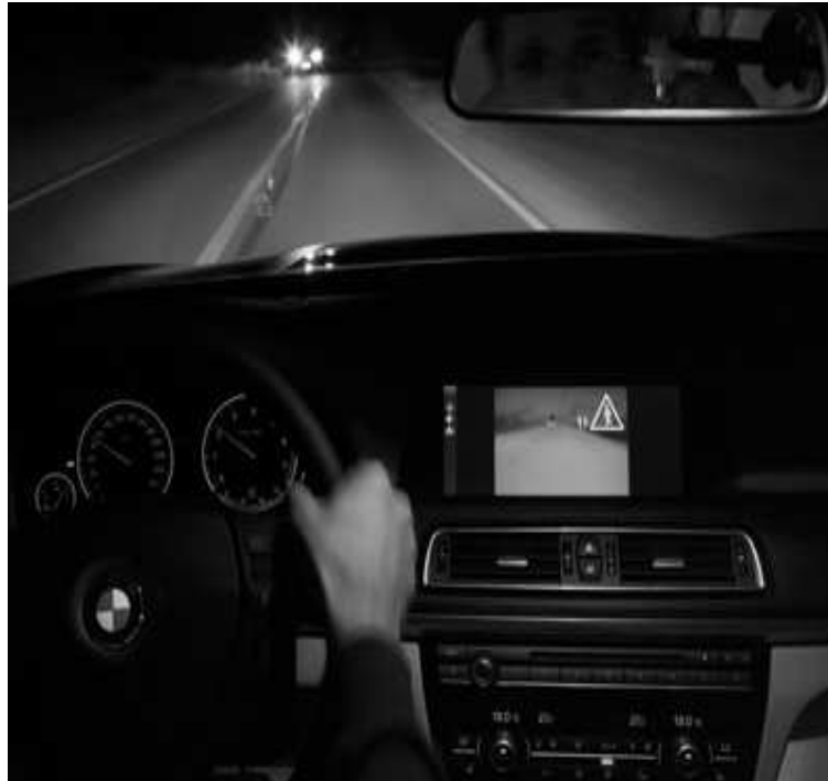
Fig. 4. The Pedestrian Protection System used in BMW cars [7]
