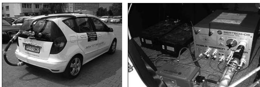
Fig. 1. View of the vehicle during the tests with the fitted SEMTECH DS analyzer
