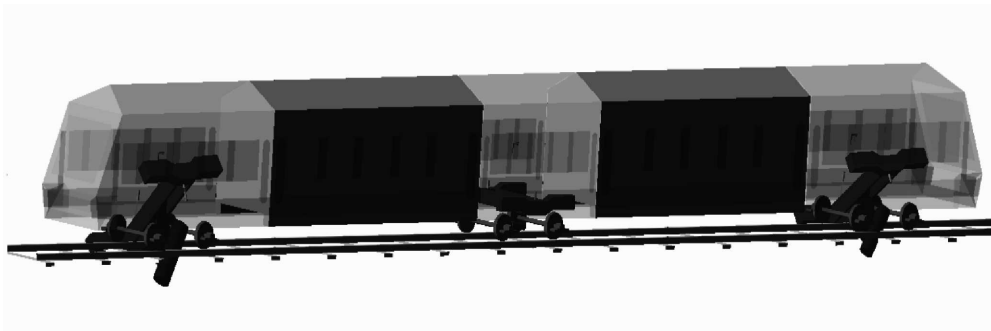
Fig. 9. Normal mode no. 32 – torsion of bogies along longitudinal axis for 14.22Hz
