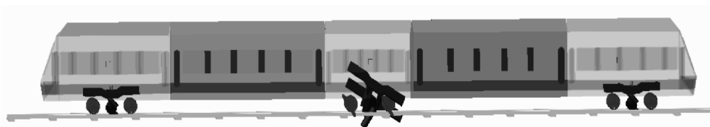
Fig. 7. Normal mode no. 19 – torsion of bogie for 10.32Hz
