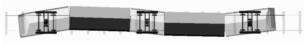
Fig. 4. Normal mode no. 2 – transversal vibrations for 0.72Hz
