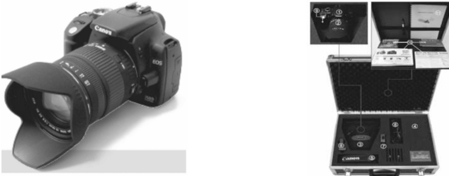
Fig. 1. The view of LMK camera for luminance measurement together with indispensable equipment [3]
