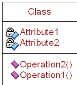
Fig. 1. Class diagram. Graphical presentation of the objects class
