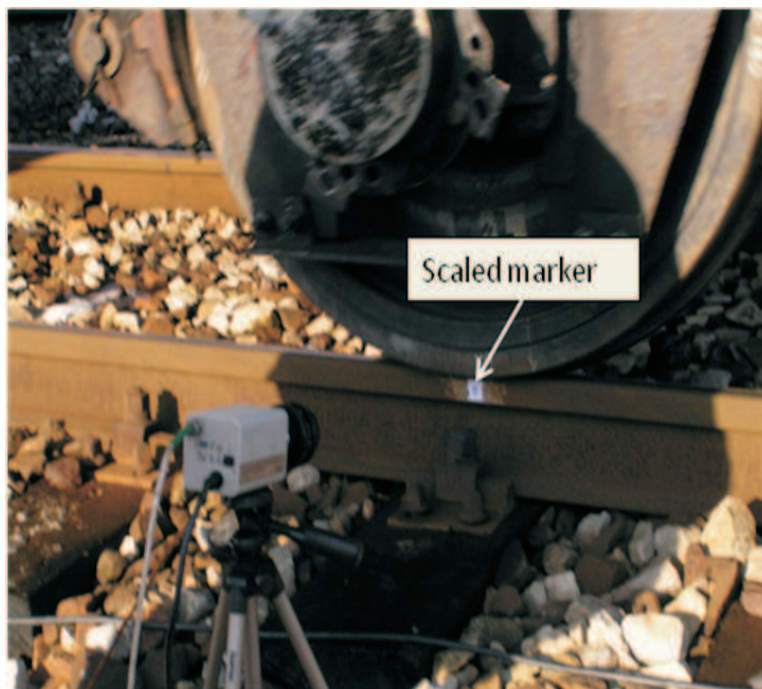
Fig. 2. View of rails with stick marker over the sleeper and the camera filming the passage
