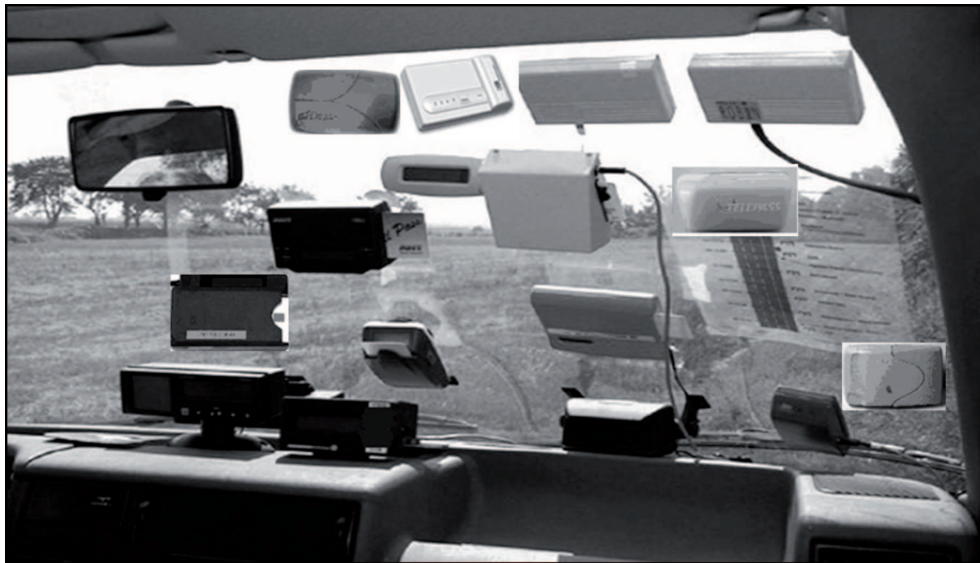
Fig. 3. Onboard OBU devices currently used on vehicles [4]
