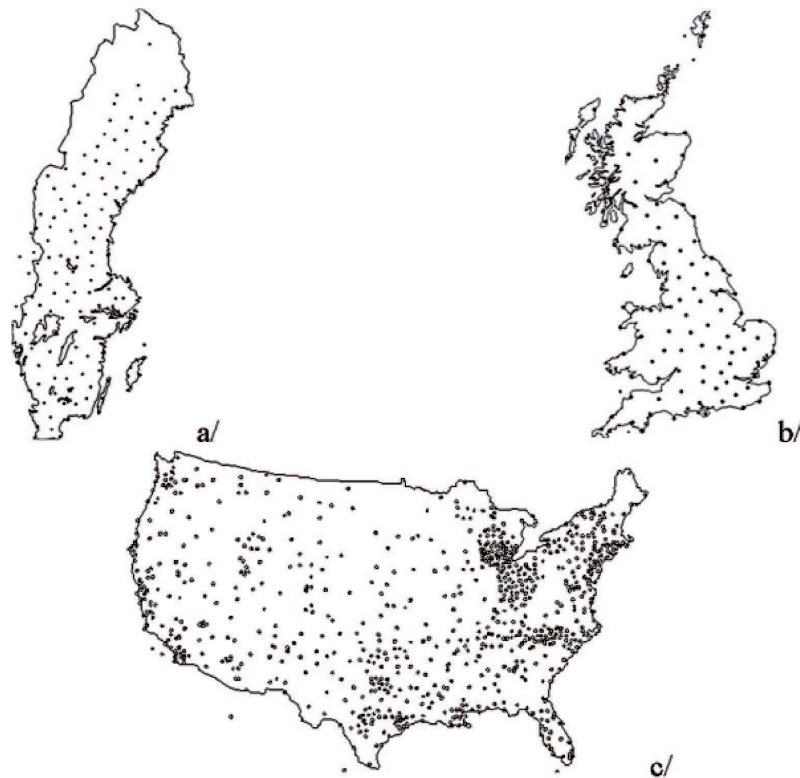
Fig. 1. Architecture of chosen active geodetic networks: a/ SWEPOS – Sweden, b/ OS-AGN – Great Britain, c/ CORS – USA
