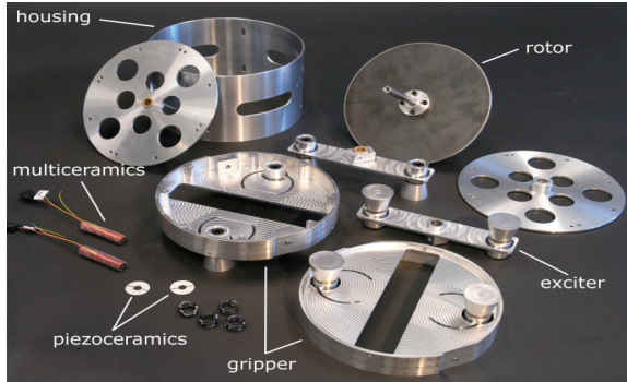
Fig. 5. Disassembled hybrid piezoelectric [6]
