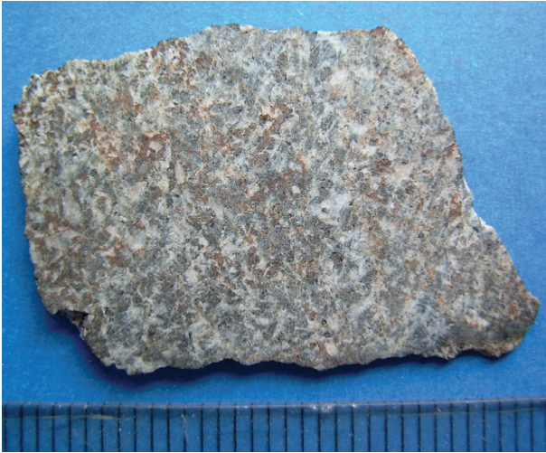
Fig. 1. Macroscopic view of the HaH 286 meteorite sample. White minerals are plagioclases, gray minerals are pyroxenes.
