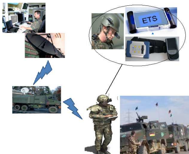
Fig. 4. The concept of the telemaintenance system in the German Land Forces to support expedient repairs during combat operations
