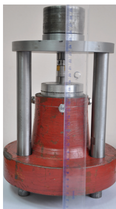
Fig. 9. The flywheel energy store
