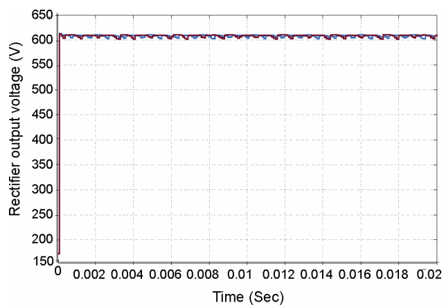
Fig. 8. Output voltage waveforms of the two parallel 18-pulse rectifiers
