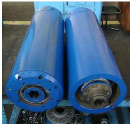
Fig. 1. General view of the specially designed induction motors in a pipe version SAR-55/1500/09 [1, 2]
