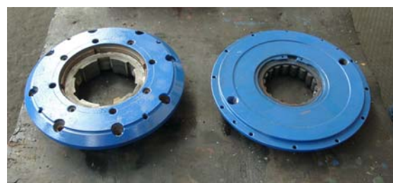
Fig. 2. The cover of slide bearing set used in the asynchronous motor SAR-55/1500/09; the bearing was made of sintered carbides of type GT-30P-5/6/11/25 [1, 2]
