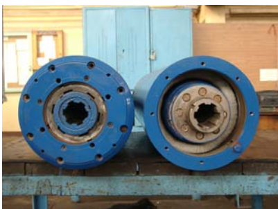
Fig. 1. A bottom of the asynchronous motors SAR-55/1500/09 with a cover of the slide bearing set [1, 2]
