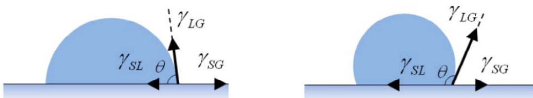
Fig. 1. Schematic view of the forces at the triple line (Solid, Liquid, Gas): a) Hydrophilic contact, \theta < 90^\circ ; b) Hydrophobic contact, \theta > 90^\circ
