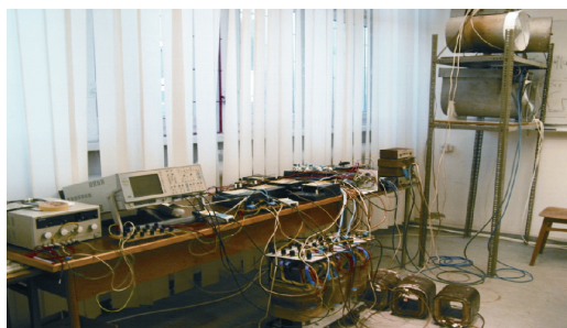
Fig. 8. Autotransformer prototype at the measurement station
