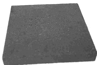
Fig. 7. Flat multipole permanent magnet width 44mm, length 44mm, thickness 5mm
