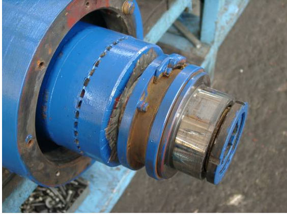
Fig. 2 Ending of the bar rotor of induction motor SAR-55/1500/09 from side of slide bearing set [1], [2]
