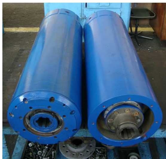
Fig. 1 A view of the pipe bodies of motors SAR-55/1500/09 [1], [2]
