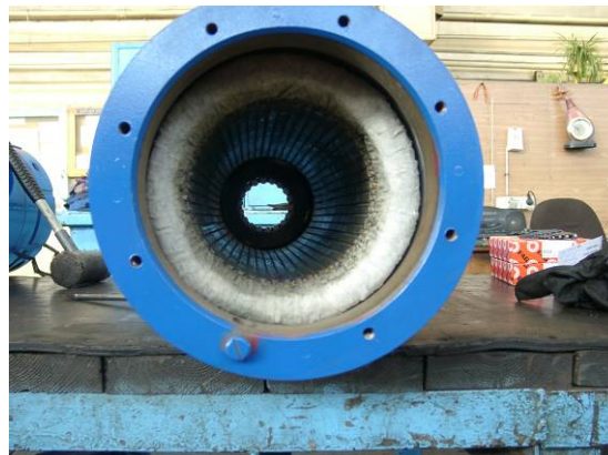
Fig. 6 Stator of motor SAR-55/1500/09 from side of slide bearing after tests in reactor with consequences of polymerization [1], [2]
