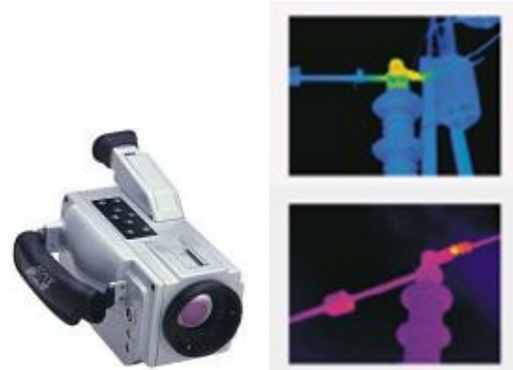
Fig. 2. Thermocamera SAT – HY 6800 and its thermograms [4]
