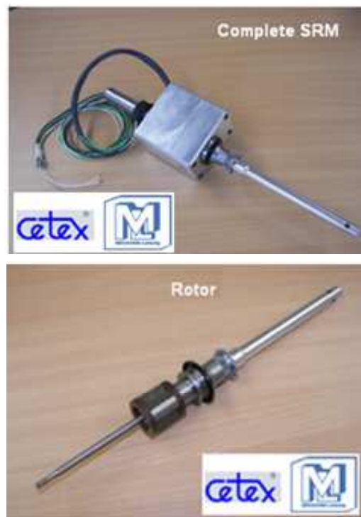
Fig. 8. Manufactured prototype of spindle-SRM
