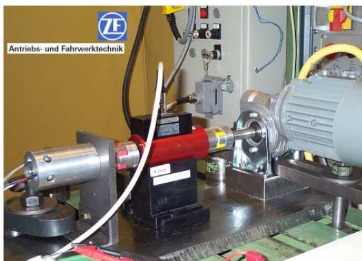
Fig 14. Gear-SRM on test bench
