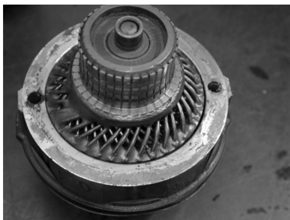
Fig. 6. Rotor of the AXIAL starter 2kW, lap winding
