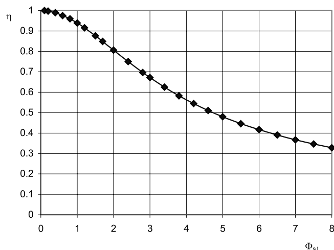
Figure 1. The relation between of \eta and \Phi_{s1} for the first order reaction
