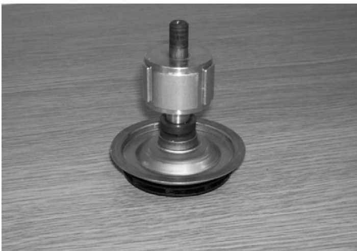
Pict. 1. The rotor with glued magnets
